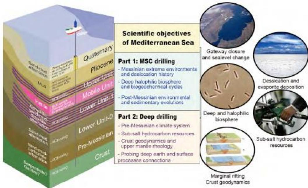
Figure 1: Conceptual image and operational plan for GOLD Mediterranean Riser drilling. Note that Part 1 is not intended to be fully cored. The first part of drilling includes some continuous as well as spot and sidewall coring in the evaporites and their immediate pre- and post-depositional units, and a second part proposed to drill and sample the section below the Messinian and down to the basement.
