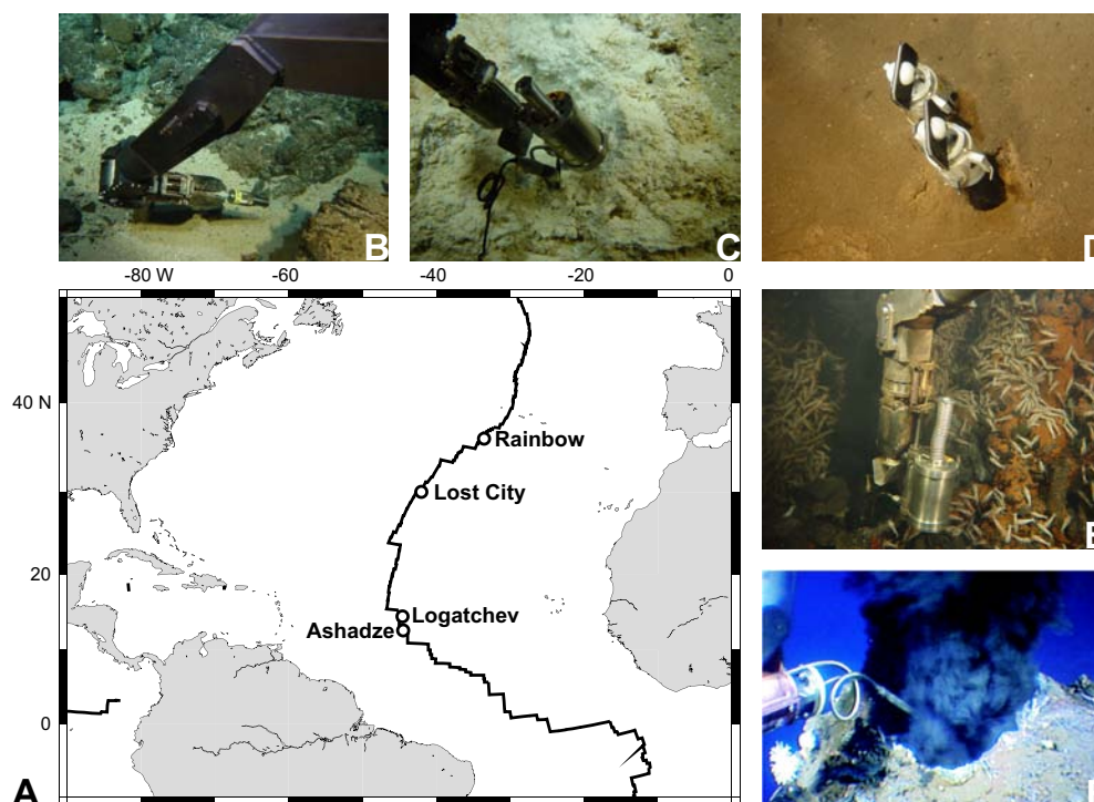
FIG. 2.17: A. Map of the location of Atlantic ultramafic sites. B. Photograph of the sediment sampling at Lost City hydrothermal field. C. Photograph of the fluid sampling using titanium syringe at Lost City hydrothermal field. D. Photograph of the sediment sampling using push-core devices at Rainbow hydrothermal field. E. Photograph of the fluid sampling using titanium syringe at Rainbow hydrothermal field. F. Photograph of temperature measurements at Ashadze 1 hydrothermal field.
