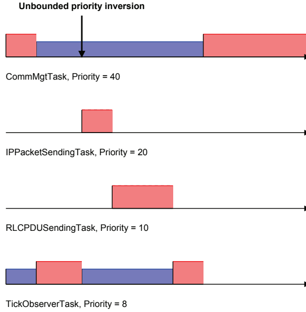
Figure 4.11: Unbounded Priority Inversion: A high rectangle means the task is executing; A low rectangle that it is preempted
