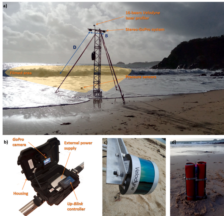
Fig. 2. a) Experimental setup showing the Stereo-GoPro system and the multi-beam laser profiler installed atop a 5.5 m tower, and the pressure sensors partly buried in sand within the shared measurement area. The photo was taken during the flowing tide. Close-up view on b) the camera system, c) the 16-beam Velodyne laser profiler, and d) the two pressure sensors attached to a sand screw.
