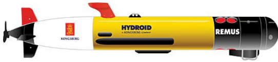
FIGURE 1. The Remus 100 AUV at the NTNU applied underwater robotics laboratory (AUR-Lab); see https://www.ntnu.no/aur-lab .
