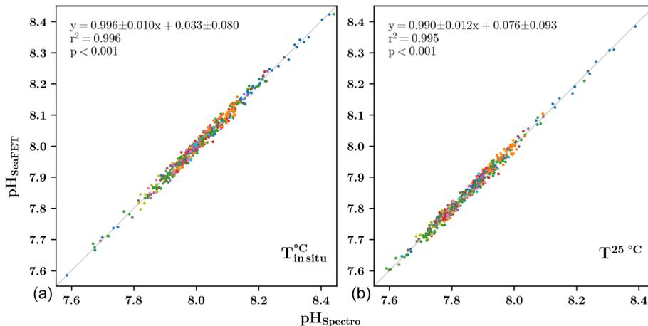
**Figure 4.** Comparison of chosen pH<sub>T</sub> (pH on the total scale) corrected SeaFET signal (pH<sub>SeaFET</sub>) versus spectrophotometric measurements (pH<sub>Spectro</sub>) at in situ temperature (a) and at 25 °C (b). The color represents a unique site and the grey line represents the 1 : 1 relationship.
