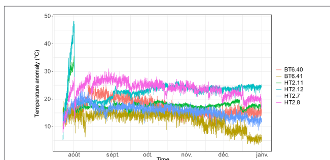
FIGURE 6 | Evolution of temperature anomaly (difference between measured temperature and background bottom seawater temperature at the site) measured with six i-buttons' temperature probes at Y3 (Lucky Strike vent field, Mid-Atlantic Ridge) from 23 July to 31 December 2014. Labels indicate probe name.
