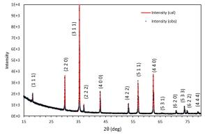
Fig. 3. XRD patterns of samples Ni<sub>x</sub>Zn<sub>y</sub>Cu<sub>z</sub>Co<sub>1-x-y-z</sub>Fe<sub>1.98</sub>O<sub>4</sub> ferrites
