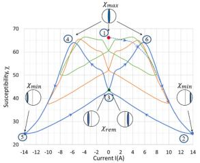
Fig. 6. Initial susceptibility measured at 10 kHz for currents up to 14 A. (In Green:  $I_{max} = 8 A$ , in Orange:  $I_{max} = 10 A$ , in blue:  $I_{max} = 14 A$ )
