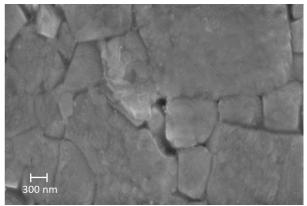
Fig. 2. SEM image of sample Ni<sub>x</sub>Zn<sub>y</sub>Cu<sub>z</sub>Co<sub>1-x-y-z</sub>Fe<sub>1.98</sub>O<sub>4</sub> ferrite
