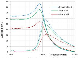
Fig. 9. Microwave susceptibility for three magnetization states. (solid lines: real part; dashed lines: imaginary part).
