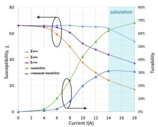
Fig. 8. Initial susceptibility and tunability measured at 10 kHz. (left scale: susceptibility; right scale: tunability).
