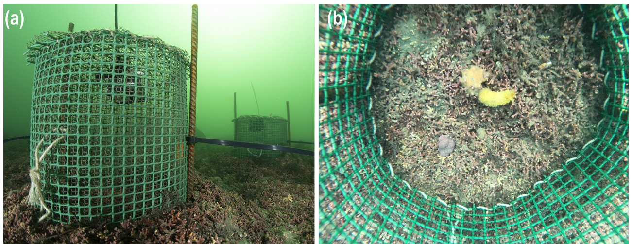
Figure 2. (a) In situ experimental setup to determine nudibranch feeding rates on the sponge Hymeniacidon perlevis in the maerl bed of Lomergat (Bay of Brest, France). (b) Top-down view of the inside of an incubation cage. The nudibranch Doris verrucosa approaches to eat the sponge H. perlevis after 30 min of incubation. Time lapse of the in situ incubation is available as Video S1.
