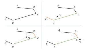
Figure 4: Closest (green) and second closest (orange) segments of a route prototype with respect to a point of interest. Top-left: a 4-segment prototype, from A to E. Top-right: classical case. Bottom-left:  $\overline{BC}$  is the second segment, because adjacent to  $\overline{CD}$  (the closest), although  $\overline{AB}$  is closer. Bottom-right:  $\overline{CD}$  and  $\overline{BC}$  are at the same distance
