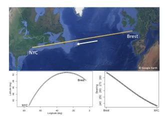
Figure 1: Illustration of the variation of the bearing along one segment. Top: geodesic line linking Brest and New York City (great circle arc). Bottom left: representation of the segment on a traditional planimetric map. Bottom right: evolution of the value of the local bearing of a mobile along the segment from Brest (start, left) to New York City (arrival, right). Angles are in degrees from the North, therefore 270 is full West.
