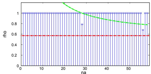
Figure 10. Estimation of the interleaver period (Hamming code)
