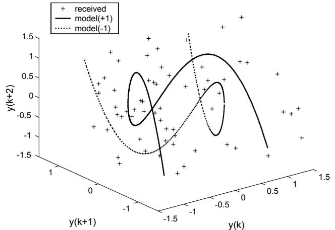
Figure 3: Representation of vectors  $\mathbf{y}_k$  and symbolic models  $\mathbf{z}_{+1}(x)$  and  $\mathbf{z}_{-1}(x)$  in a 3-dimensional space ( $N = 3$ ). The map is  $g(x) = 1 - 2x^2$  and the signal to noise ratio is  $SNR = 3dB$ .
