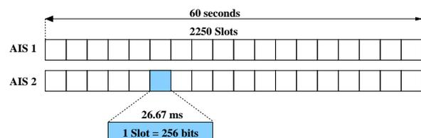
Figure 1: AIS frame organization in TDMA mode
