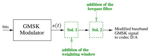
Figure 2: Proposed solutions to avoid AIS interference
