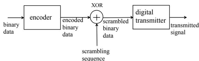
Figure 1: Principle of scrambling
