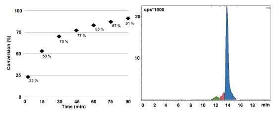
**Figure 3**. <sup>1</sup>H NMR spectroscopic monitoring of maleimide coupling reaction on GluCAB-2<sup>NH2</sup> (left). Radio-HPLC chromatogram of [<sup>64</sup>Cu]Cu-GluCAB-2<sup>Mal</sup> (right).
