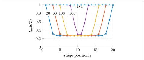
**Fig. 7** Convergence of the binary SC-CPM stages as function of the decoding iterations (number above the lines) at  $E_5/N_0 = -2.58$  dB. Here, L = 20
