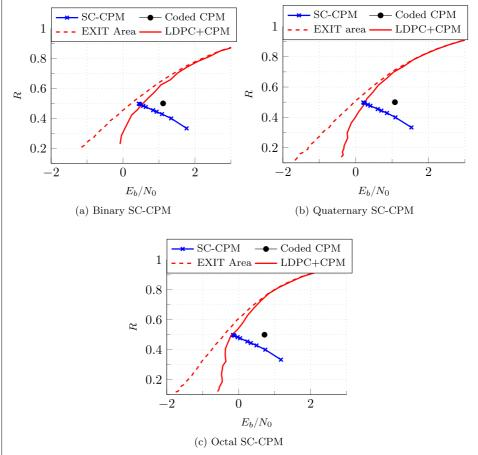
**Fig. 8** Threshold of coupled and uncoupled coded CPM. Comparison to the area under the EXIT is also depicted. The coupling matrix here is  $B = [\frac{1}{2}, \frac{1}{2}]$
