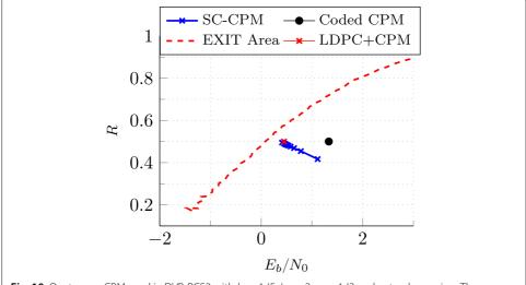
**Fig. 10** Quaternary CPM used in DVB-RCS2 with  $h=1/5, L_c=2, \alpha=1/3$  and natural mapping. The coupling matrix is always given by  $B=[\frac{1}{2},\frac{1}{2}]$
