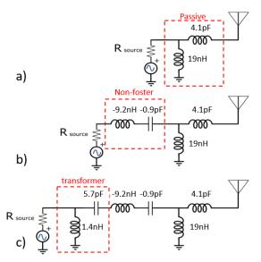
**Fig. 15** Illustration of the step-by-step matching using the 3<sup>rd</sup> topology (a) Passive matching, (b) Non-Foster matching, (c) Passive transformer
