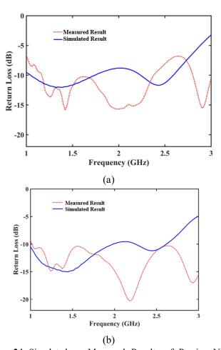
**Fig. 24** Simulated vs Measured Results of Passive NF matching of second topology (a), and third topology (b)
