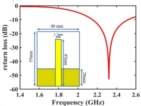
Fig. 1 Antenna schematic and return loss
