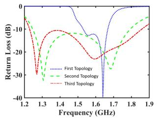
Fig. 17 Comparison of the return loss from the three topologies
