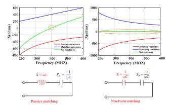
**Fig. 5** Comparative concept of passive and NF matching for an ESA modeled by a series capacitor.
