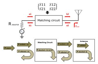
Fig. 19 Incident and reflected waves at the matching circuit accesses
