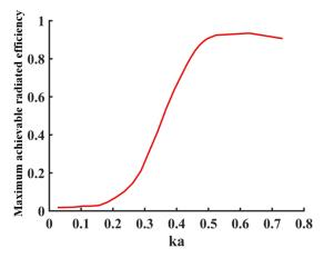
Fig. 3 Maximum achievable antenna radiation efficiency
