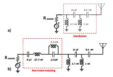
**Fig. 8** Antenna with Passive transformer (a), antenna with NF-Passive matching (b)
