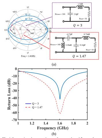
**Fig.4** Comparison between 1 stage L-network and 2 stage L-network on Q factor (a), the effect of Q factor on bandwidth for a  $5\Omega$  load.
