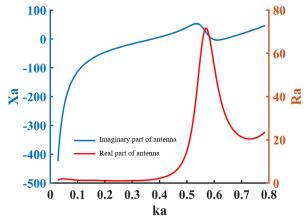
Fig.2 Antenna impedance (real and imaginary) parts
