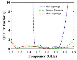
Fig. 18 Comparison between Q factor of the whole matching network of the three topologies
