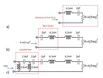
Fig. 12 Antenna model at low frequency (a), NF reactive part compensation (b), complete matching (c)
