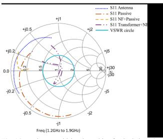
Fig. 16 Step-by-step wideband matching for the 3rd topology
