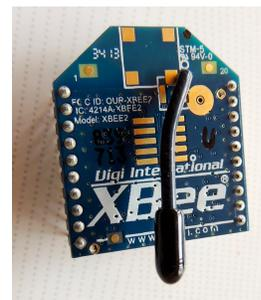
Figure 4. Radio module with pinout for serial control and data acquisition. Such modules can emit from few meters to kilometers depending on standards. They can fit Arduino boards
