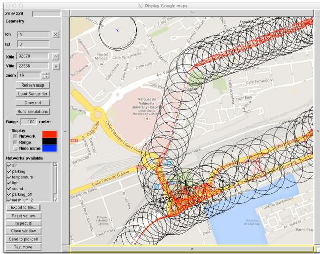
Figure 6. 1<sup>st</sup> generation browser displaying the Smart Santander european sensor experiment in real-time. 7 different networks are displayed which sensor connection range is tuned to 100meters. This browser is able to produce simulation architectures and to present data from simulation processes
