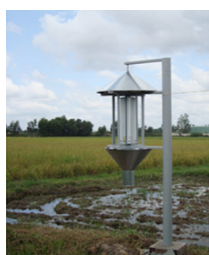
Figure 1. A light trap beside a rice field. Top to bottom are a cover to protect from rain fall, a low energy bulb, glasses that are illuminated, a basin with water (sometimes insecticide) to kill insects. In this case, the power come from a farmer house close to the trap.
