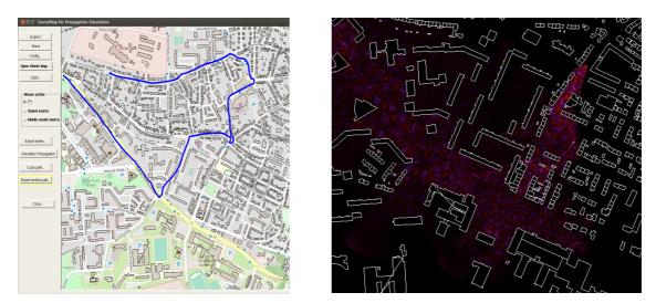
Figure 1. Simulation of siren alert along an emergency vehicle path. The left figure is part of a city map, with a trip path used by many health transport vehicles having sirens. The right part displays a sample of sound pressure estimation in part of this path. Red pixels represent expected sound on city locations.
