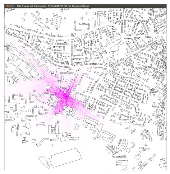
Figure 4: Graphical representation of cellular automata running. The dark lines show the wall of the buildings and other obstacles. This allows us to account for the complexity of buildings topology as encountered in urban areas.
