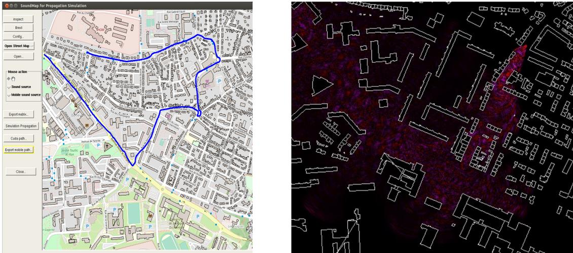
Figure 1. Simulation of siren alert along an emergency vehicle path. The left figure is part of a city map, with a trip path used by many health transport vehicles having sirens. The right part displays a sample of sound pressure estimation in part of this path. Red pixels represent expected sound on city locations.
