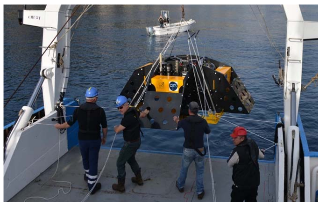
Fig. 1. Deployment of a MUG-OBS (2.9m x 2.9m x 1m, for a weight in Air of 1.5t (3307Lb)). The frame is made of non-conductive material (syntactic foam, polyethylene, glass and titanium cases) and shaped to resist trawling.
