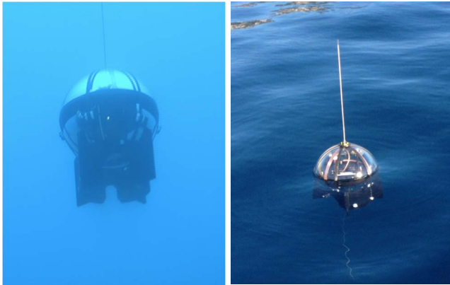
Fig. 3. Data shuttle on its way to the surface and at sea-surface. The electronic, encapsulated in a 13'' glass sphere, is designed around a Cortex M4 microprocessor, memory boards (SD cards), an internal clock, a flash light, a GPS and AIS to track the shuttle on the surface, and is powered by a Lithium battery. The shuttle clock synchronizes with the main clock of the system prior to its release, and synchronizes itself as soon as a GPS signal is received at sea-surface. This enables monitoring the clock-drift of the main acquisition clock at every shuttle recovery over the 3 years of the MUG-OBS deployment.
