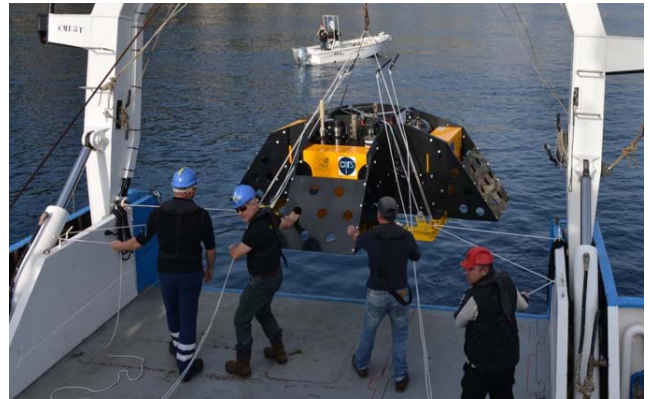
Fig. 1. Deployment of a MUG-OBS (2.9m x 2.9m x 1m, for a weight in Air of 1.5t (3307Lb)). The frame is made of non-conductive material (syntactic foam, polyethylene, glass and titanium cases) and shaped to resist trawling.
