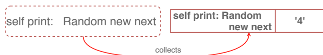
Figure 2: A collector: the dotted line represents the target AST node (on the left), while the resulting object is stored each time it is evaluated at runtime (on the right).
