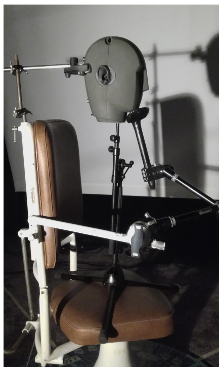
Fig. 3. Position of the dummy head, maintained by the headrest and chin rest, during the recording of the stimuli.
