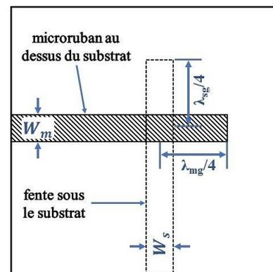
Figure 1. Transition microruban-ligne fente
