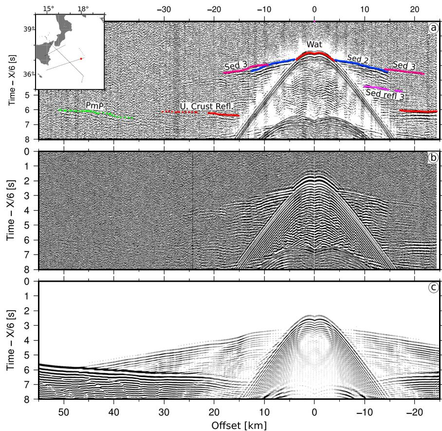
**Figure 5.** Seismic section of the ocean bottom seismometer (OBS) 48 on DYP1 profile. (a) Interpretation of the seismic section preprocessed with annotation of each phases identified: Wat (for Water reflection arrival), sed 2 (for sediments), sed 3 (for deeper sediments), U. Crust Refl. (for upper-crustal reflections), and PmP (for Moho reflection phase). (b) Raw seismic section of OBS 48. (c) Synthetic arrivals calculated from the velocity model. And location map of the OBS.
