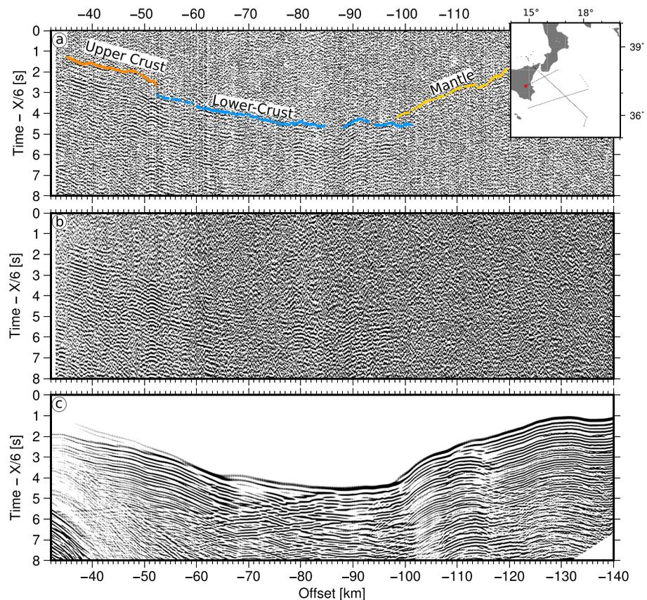
**Figure 2.** Example of the data acquired by the land station 6 of the northern DYP3 profile. (a) Interpretation of the seismic section preprocessed with annotation of each phases identified: upper crust, lower crust, and Mantle refraction phases. (b) Raw seismic section of the land station 6. (c) Synthetic arrivals calculated from the velocity model with location map of the station.
