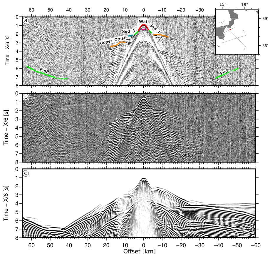
**Figure 3.** Seismic section of the ocean bottom seismometer (OBS) 10 on DYP3 profile. (a) Interpretation of the seismic section preprocessed with annotation of each phases identified: Wat (for Water direct arrival), Sed 1 (for Shallow sediments), sed 2 (for deeper sediments), and upper-crustal refraction phases. (b) Raw seismic section of OBS 20. (c) Synthetic arrivals calculated from the velocity model. And a location map of the OBS observed.
