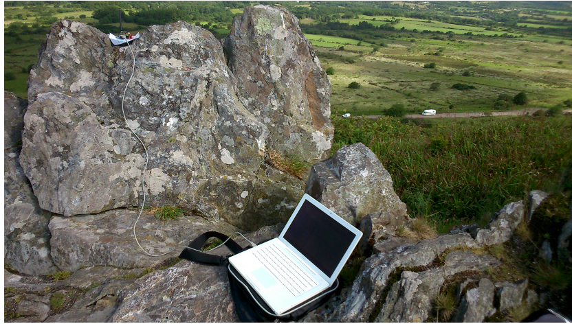
Figure A5. A base station is equipped with a LoRa board (emitter) and a MacBook. This base station was deployed on the top of the Roc’h Trevezel mountain, France. The receiver is another LoRa board mounted on a car moving around.
