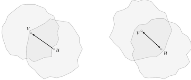
(a) Asymmetrical link due to the radio irregularity ( u can hear v but not vice versa). (b) Symmetrical link ( u can hear v and vice versa).
