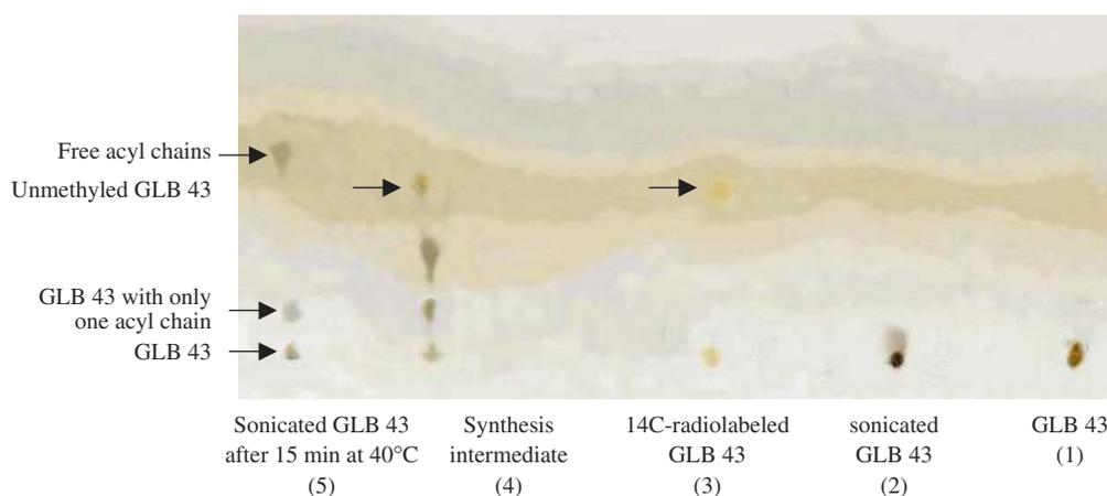
**Figure 3. Chromatogram obtained after migration of GLB43 samples differentially treated. Each sample was applied onto a silica gel plate. The chromatogram was developed to 10 cm using ethanol, and then revealed**
