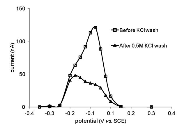
Fig. 4. AC voltammograms recorded at a frequency of 24 Hz for cyt *c* immobilized on a CL/PC-modified electrode before (open squares) and after (open triangles) washing with 0.5 M KCl solution.
