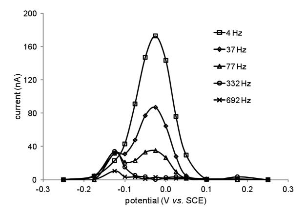
Fig. 3. Representative AC voltammograms recorded at frequencies ranging from 4 to 692 Hz for cyt c immobilized on a CL/PC-modified GC electrode in a 20 mM TRIS-HCl buffer solution (pH 7). Data are background corrected.
