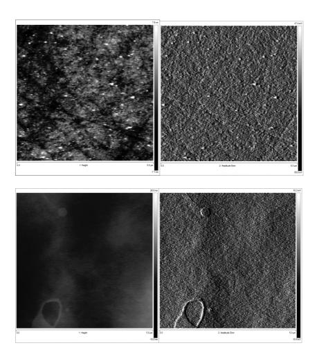
Fig. 1. Topographic (left) and error amplitude (right) AFM images. Same spot on the electrode before (A) and after (B) deposition of a CL/PC film. Small patches of bilayer characterized by a relative height of 2 nm can be observed at the bottom left.
