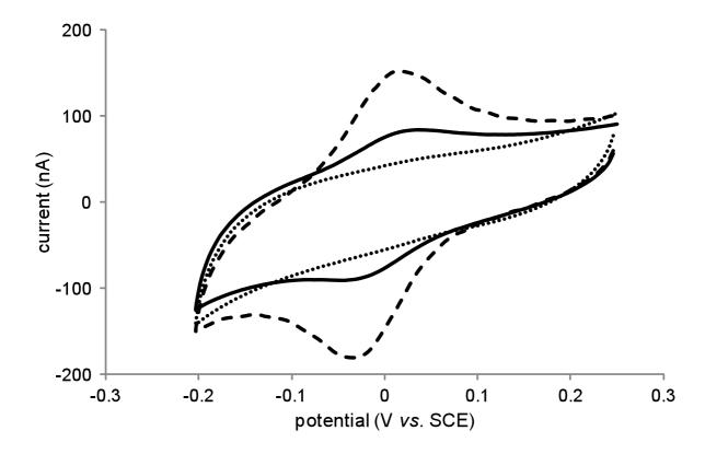
Fig. 2. Representative examples of voltammograms recorded at a bare GC electrode (dotted trace) and a CL/PC-modified GC electrode (dashed trace) in a solution containing 50  $\mu$ M cyt c and 20 mM TRIS-HCl (pH 7). The voltammogram recorded for the same lipid-modified GC electrode after transfer in a 20 mM TRIS-HCl buffer solution that does not contain cyt c is also shown (solid trace).
