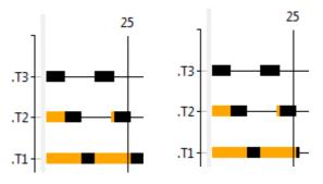
At tick 25 indeed, *Thread* T1 should start a new period, but it cannot happen as it is still preempted by T2 at that time and has not completed its previous job. With the current implementation of the two tools, Cheddar (on the left) starts the new job of T2 even if late, whereas Marzhin (on the right) skips the missed job. Further investigation would be required to determine which of these two behaviors is the more realistic according to actual RTOS implementations.
