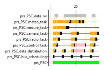
We can observe that some high priority *Threads* are postponed by low priority *Threads* that are blocking the access to the shared *Data*. The priority inversion phenomena is highlighted by the fact that the high priority *Threads* are in a "wait for resource" state
