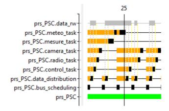
Note that the *Threads* are shown with an increasing level of priority (i.e. the bus scheduling *Thread* has the highest priority). If the PCP concurrency protocol is removed from the shared *Data* component, the "priority inversion" problem is displayed by Marzhin as follows:
