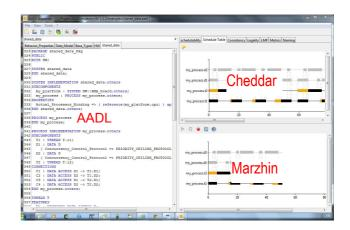
This verification approach is of course limited by the fact that Cheddar cannot provide a significant result for any kind of AADL architecture. However, it must be recalled that the role of Marzhin is specifically to complement Cheddar with cases that cannot be processed in a deterministic manner.
