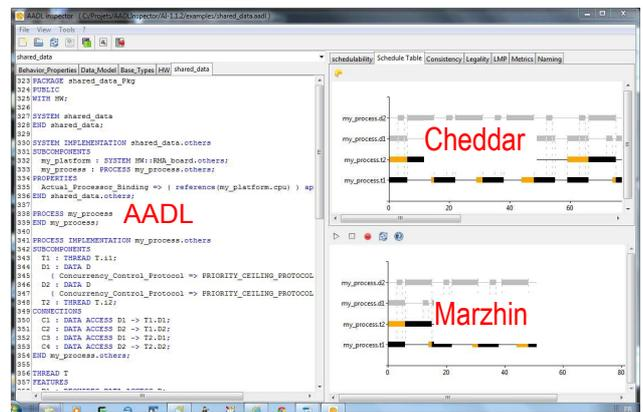
This verification approach is of course limited by the fact that Cheddar cannot provide a significant result for any kind of AADL architecture. However, it must be recalled that the role of Marzhin is specifically to complement Cheddar with cases that cannot be processed in a deterministic manner.
