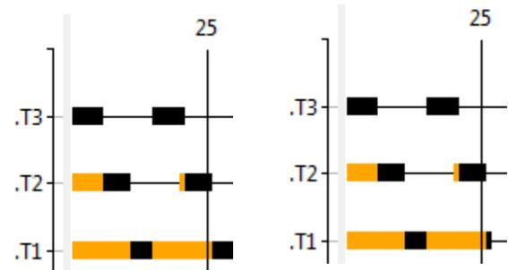
At tick 25 indeed, *Thread* T1 should start a new period, but it cannot happen as it is still preempted by T2 at that time and has not completed its previous job. With the current implementation of the two tools, Cheddar (on the left) starts the new job of T2 even if late, whereas Marzhin (on the right) skips the missed job. Further investigation would be required to determine which of these two behaviors is the more realistic according to actual RTOS implementations.
