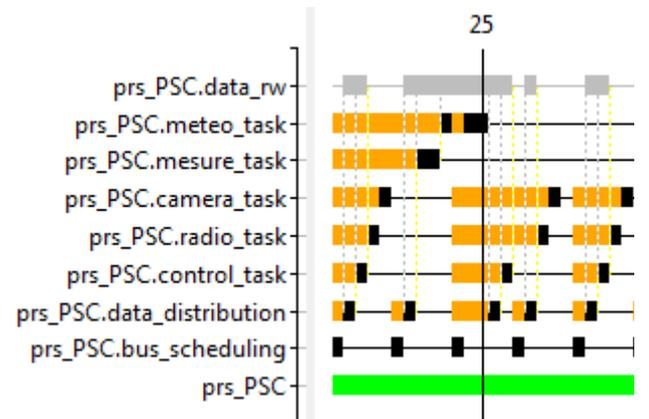
Note that the *Threads* are shown with an increasing level of priority (i.e. the bus scheduling *Thread* has the highest priority). If the PCP concurrency protocol is removed from the shared *Data* component, the “priority inversion” problem is displayed by Marzhin as follows:
