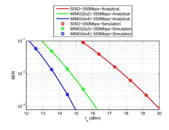
Fig. 3. 256-PPM in log-normal channel using PIN at background noise (0 dBm) for the same data rate.
