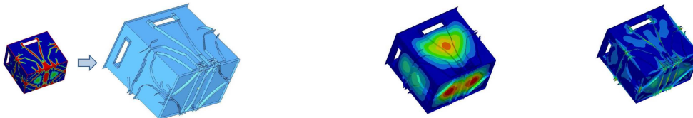
Figure 4: from the left to the right, the distribution of stress, the resulting ribs, the displacements, the von Mises stresses
