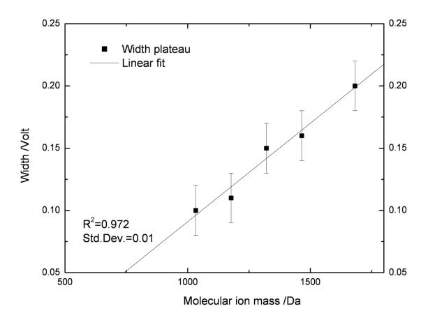
**<u>Fig. 4:</u>** Width of the plateau (intermediate excitation regime) as a function of molecular ions mass for a mixture of  $[PLA_n+Li]^+/[PTMEG_n+Li]^+$ . Details on calculations and estimation of error bars are presented in the text.
