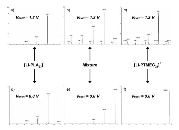
**Fig. 1:** MS/MS spectra for [PLA<sub>23</sub>+Li]<sup>+</sup> (spectra a and d), [PTMEG<sub>23</sub>+Li]<sup>+</sup> (spectra c and f) and a 5:1 mixture (spectra b and e), obtained at 0.8 Volt (spectra d, e and f) and 1.3 Volt (spectra a, b and c) excitation voltages.
