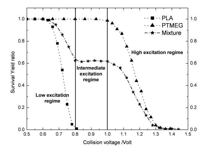
**Fig. 2:** Survival Yield curves for [PLA<sub>23</sub>+Li]<sup>+</sup> (filled squares with dotted line) and [PTMEG<sub>23</sub>+Li]<sup>+</sup> (filled triangles with dotted line) and a 5:1 mixture of [PLA<sub>23</sub>+Li]<sup>+</sup>/ [PTMEG<sub>23</sub>+Li]<sup>+</sup> (filled stars with dot dashed line).
