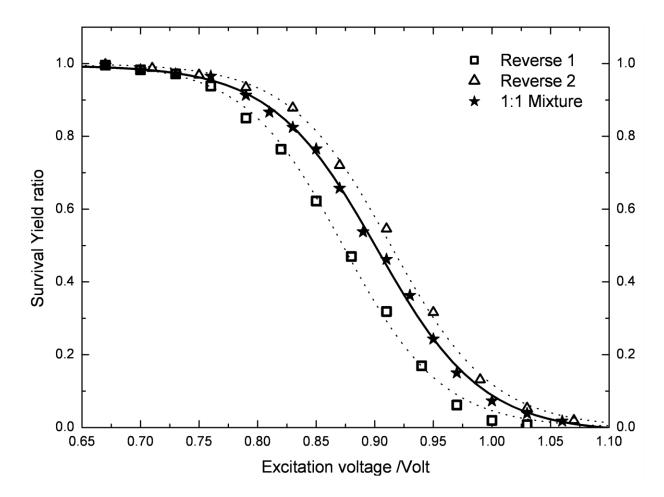
**Fig. 5:** Survival Yield curves for two protonated peptides with inverted sequences at m/z 708.3: H-(SDGRGAF)-NH<sub>2</sub> (reverse 1) and H-(FAGRGDS)-NH<sub>2</sub> (reverse 2). SY curve for a 1:1 mixture is also presented.
