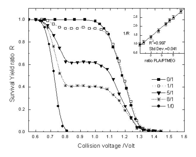
**Fig. 3:** SY curves for PLA/PTMEG mixtures at relative concentrations 0:1, 1:1, 5:1, 8:1 and 1:0, in the same experimental conditions. The inset shows the correlation between the inverse of the
