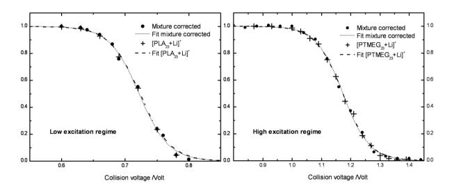
**Fig. S-1:** SY curves were obtained with pure homopolymers (crosses) of [PLA<sub>23</sub>+Li]<sup>+</sup> (left) and [PTMEG<sub>23</sub>+Li]<sup>+</sup> (right) and a 5:1 mixture of PLA/PTMEG (filled circles on both spectra). Peaks intensities for the mixture were corrected using Eq. S-1 in the low regime (left) and using Eq. S-2 in the high regime (right). Curves were fitted using sigmoid functions (dashed lines).
