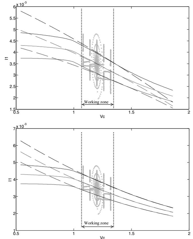
Fig. 3a and 3b. Solid lines: static characteristics of a commercial driver: output current  $i_1$  versus common mode voltage  $v_c$  for different values of the differential voltage  $v_d$ . Dashed lines: characteristics of the uncorrected (3a) and corrected (3b) models. Grey stars: values used in the identification signals.
