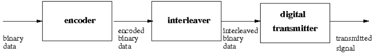
Figure 1. Principle of a digital transmission chain
