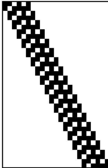
*Figure 4. Graphical representation of  $G$  to encode 18 bits*
