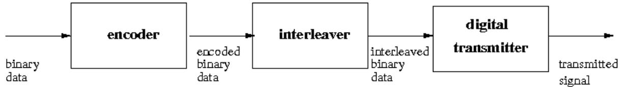
*Figure 1. Principle of a digital transmission chain*
