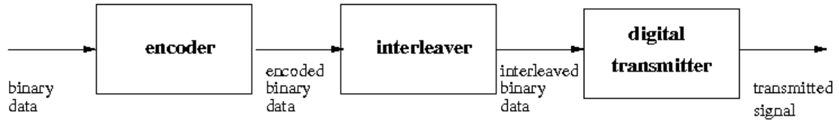
Figure 1. Principle of a digital transmission chain
