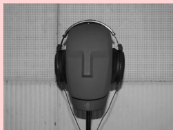
Recording of sequences played on headphones in the ears of the KU 100 dummy head.
