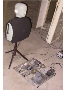
Figure 1: Acoustic dummy head placed near the test bench in order to record the 18 samples according to the experiment table.
