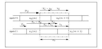
Figure 1. Relative positions of signals and an analysis window before the synchronization process,  $\,N_u^i=2$  in uplink.
