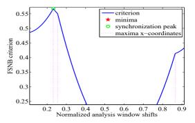
Figure 3. FSNB Criterion: case of the masking of synchronization peaks,  $N_u^i=4$
