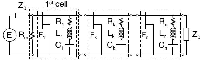
Fig. 2. Structure of the n-stages cascaded ideal circuit.
