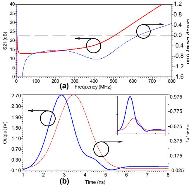
Fig. 7. Simulated S<sub>21</sub> parameter and group delay (a). Time-domain simulations (b).  $R_m = 75 \Omega$ ,  $R_1 = R_2 = 10 \Omega$ ,  $R_3 = 18 \Omega$ ,  $R_4 = 30 \Omega$ ,  $C_1 = 150 \text{ nF}$ ,  $C_2 = 3.9 \text{ nF}$ ,  $C_3 = 11 \text{ pF}$ ,  $C_4 = 2.7 \text{ pF}$ ,  $L_1 = L_2 = 3.6 \text{ nH}$ ,  $L_3 = 8.7 \text{ nH}$ ,  $L_4 = 8.2 \text{ nH}$ .
