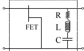
Fig. 1. Series RLC resonant network in cascade with a FET.
