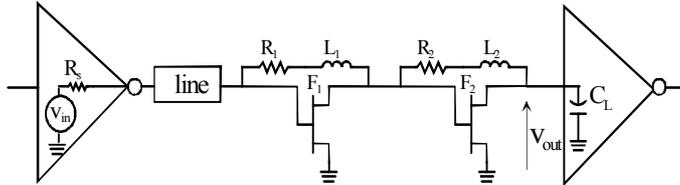
Fig. 5: Combination of the output gate ( $R_S = 90 \Omega$ ), the RLC model line with a two-stage active NGD circuit ( $F_1 = F_2 =$  FET EC2612,  $R_1 = 73 \Omega$  and  $L_1 = 99 \text{ nH}$ ,  $R_2 = 102 \Omega$  and  $L_2 = 17 \text{ nH}$ ) loaded by the input capacitor  $C_L = 30 \text{ pF}$  of the next gate.
