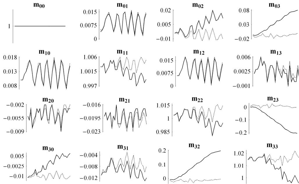
Fig.4: Evolution of the Mueller coefficients of a no-sample measurement (vacuum) versus temperature over the first 15 minutes of experiment of Fig.3. Solid curves represent Mueller coefficients with no correction, and dashed curves show them after correction by  $\phi_w$ .
