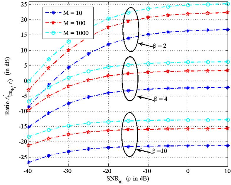
**Figure 8.**  $\Delta'_{(m_{\phi_i}, \eta)}$ ,  $\alpha = 5$ ,  $N_u^i = 30$ ,  $L_i = 511$ ,  $W = 200$  MHz,  $T_c = 150$  MHz,  $F_e = 300$  MHz.
