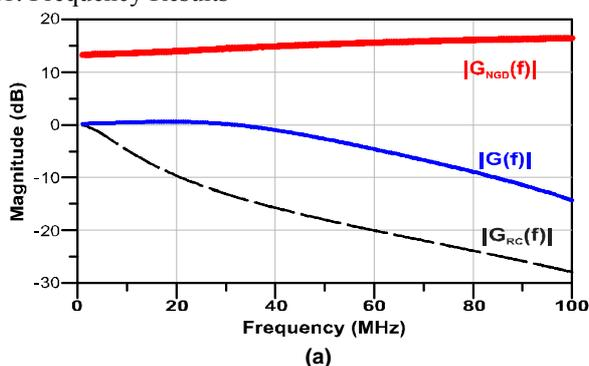
Fig. 5(a). Measured magnitudes of the RC-, NGD- and RCNGD-circuits.
