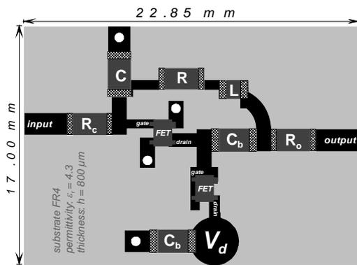
Fig. 4. Layouts of the tested RCNGD-circuit using a PHEMT ATF-34143 ( $V_{gs} = 0\text{V}$ ,  $V_d = 3\text{V}$ ,  $I_d = 110$  mA), for  $R_c = 33 \Omega$ ,  $C = 680$  pF, and  $R = 56 \Omega$ ,  $R_o = 10 \Omega$ ,  $L = 220$  nH,  $C_b = 100$  nF.
